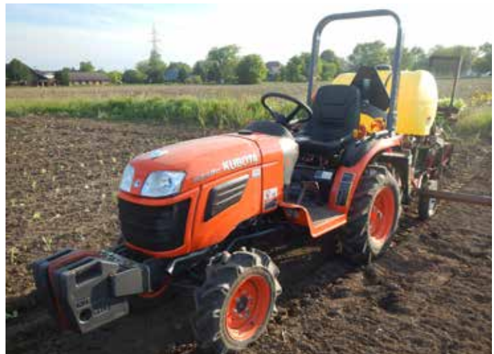
The new addition to the farm with the old transplanter. The weights in the front balance the weight of the transplanter and the person riding on the transplanter. This system makes for more efficient, easier transplanting.
